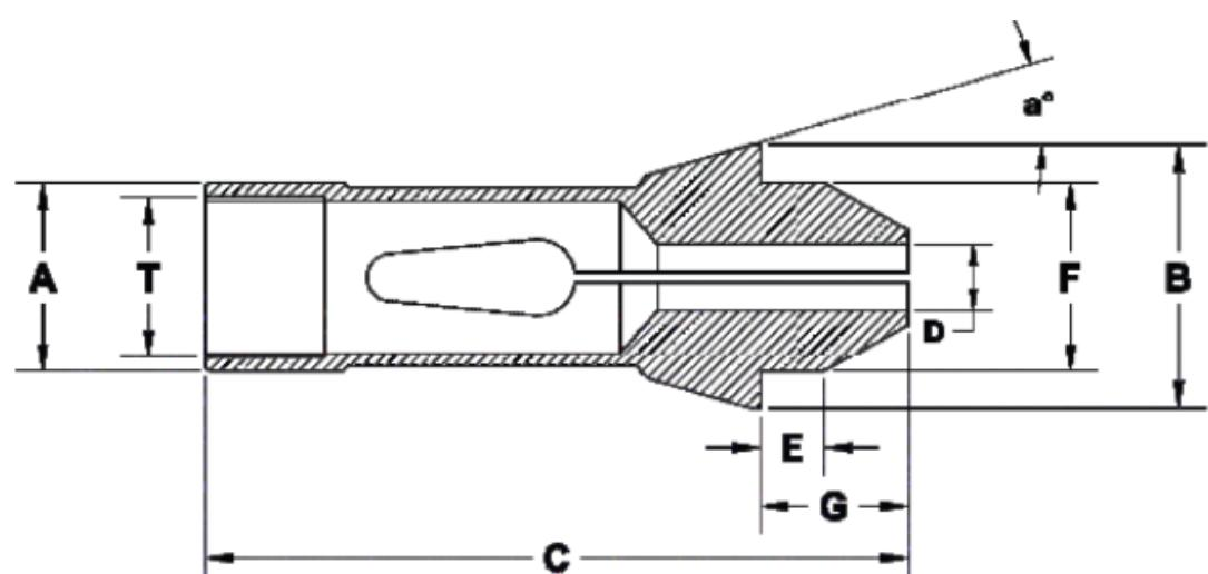
**A** Shaft - Ø   **B** Head - Ø   **F** Nose - Ø   **D** Bore - Ø   **E** Nose Length   **G** Nose Total Length
