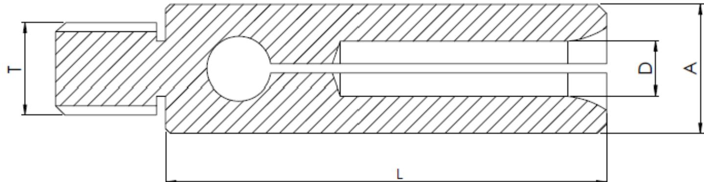
A Head-  $\varnothing$  T Thread -  $\varnothing$  L Total Length D Bore -  $\varnothing$
